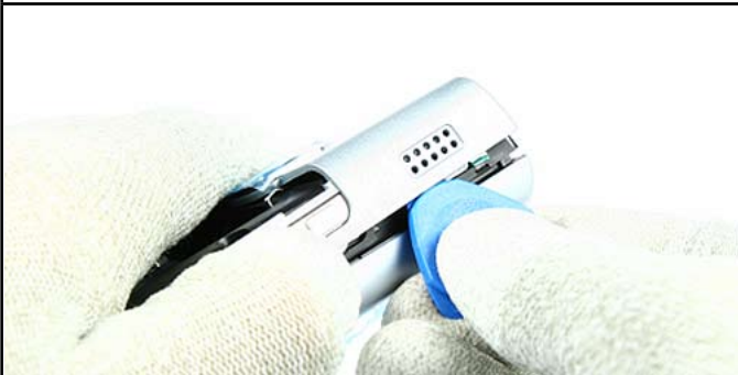
13. Release the clips of the Back Cover Assy on both sides as shown.
