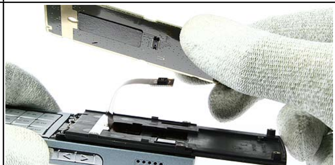
24. Remove the Upper PWB.
