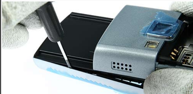
11. Release the clips on the opposite side, too.
