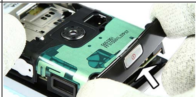
20. Remove the Top Cover Assy.
