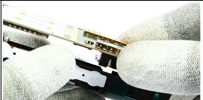
26. Lift out the Engine Module and place it into the rework jig.
