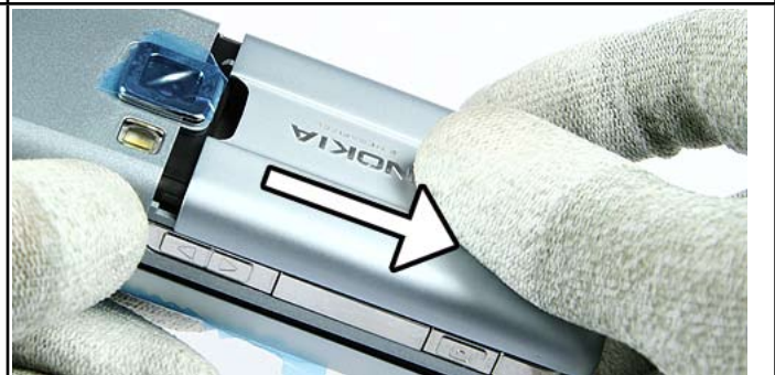
4. Remove the Battery Cover. Ensure that no battery is inserted.
