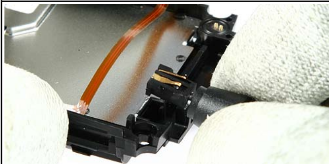
31. Remove the DC-Jack with the DC plug.
