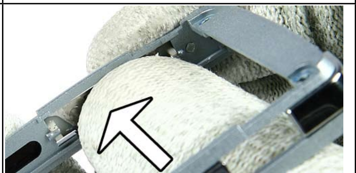
16. Carefully push out the hinge from the SD Door at the shown side first.
