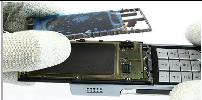
20. Remove the LCD Frame Assy.
