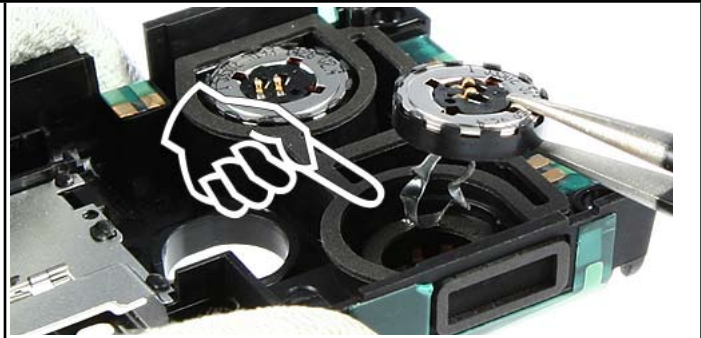
34. The IHF Speaker Adhesives will be destroyed.
