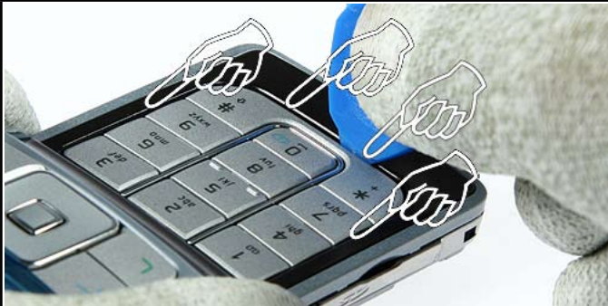
5. Release the clips of the Keymat with the SRT-6 as shown.
