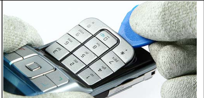
6. Ensure that all clips are released.
