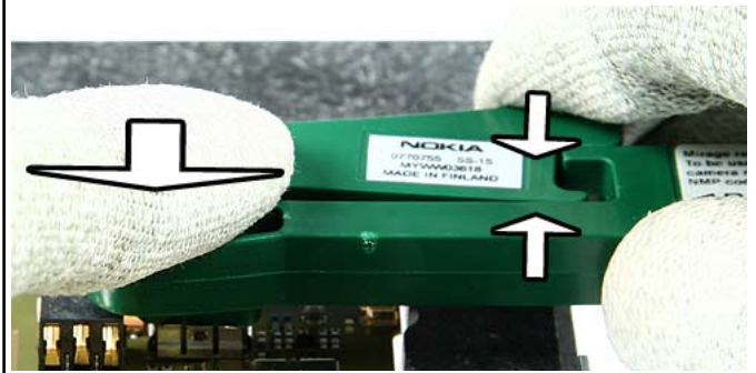
28. Place the tool and push it down carefully. Fix the Camera.
