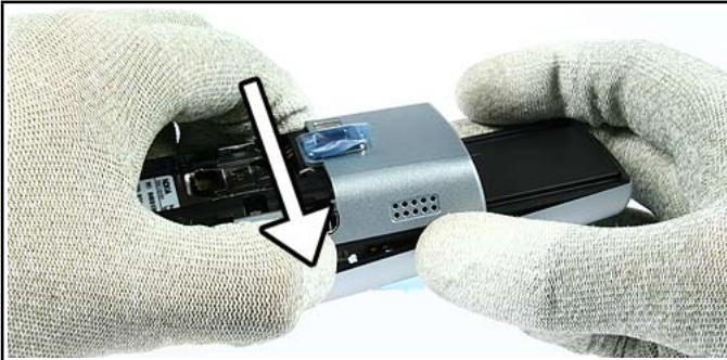
9. Now lift the lower side and hold it in this position.
