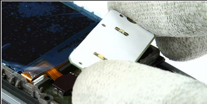
17. Remove the UI PWB.
