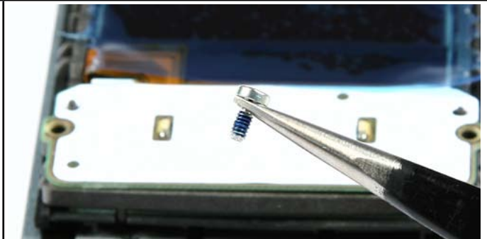
16. All screws in this phone must be renewed after removal.
