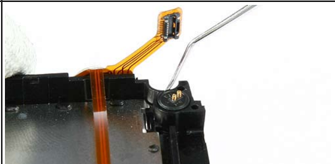
32. Remove the Microphone with the dental tool.
