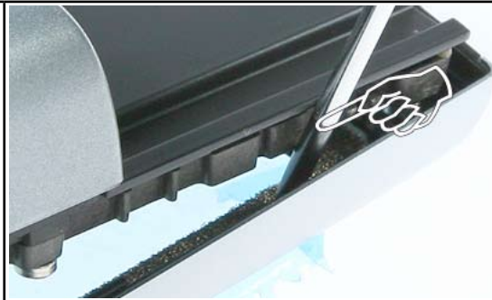
10. Carefully release the upper clips of the A-Cover with a slotted screwdriver.
