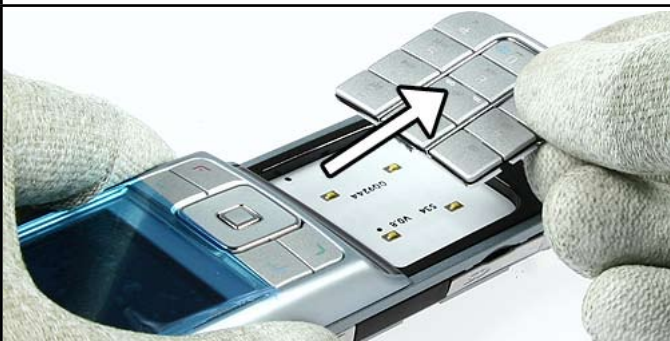
7. Separate the Keypad.
