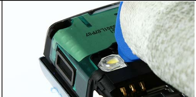
18. Release the Flash Light with the SRT-6.
